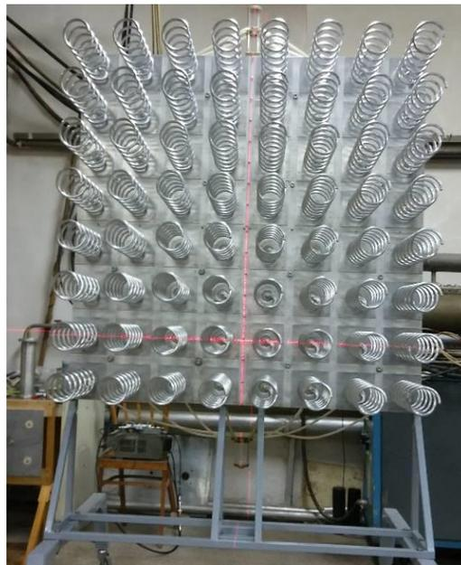
Fig. 1. The 8×8 array of cylindrical helical antennas.
