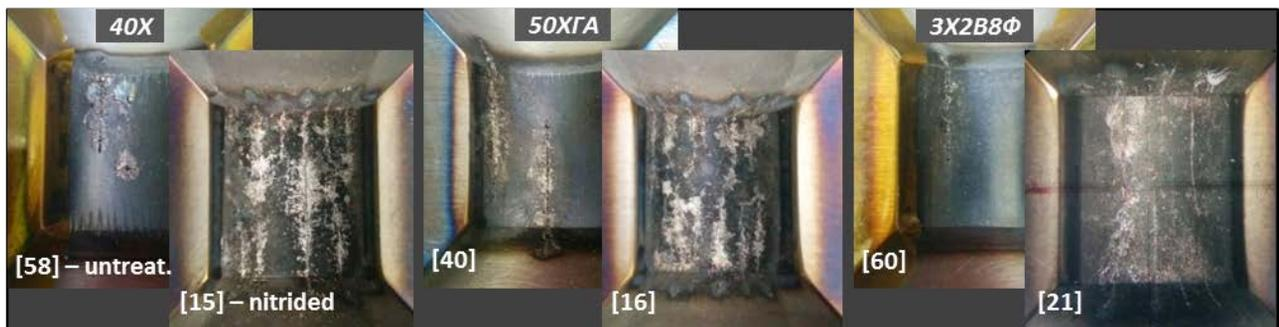
Fig. 1. Inner channel view of nitrided and without plasma treatment inductors after testing ( $B=50$  T). Durability is in brackets.
