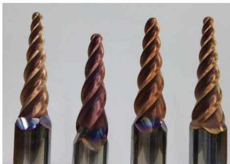
Fig 1. conical end mills with obtained coatings based on intermetallides of the Ti-Al system synthesized in the oxygen environment by vacuum arc plasma.
