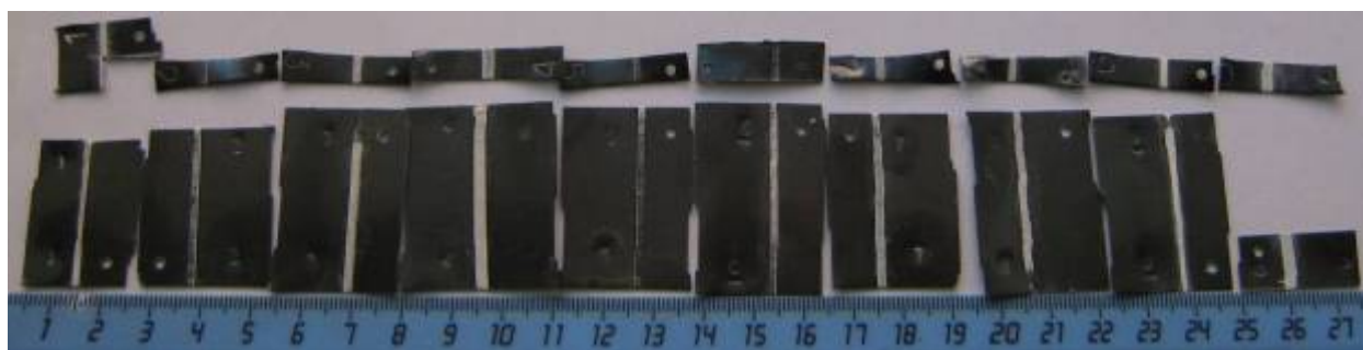
Figure 1. Samples after corrosion test (top – irradiated; bottom – without irradiation)
